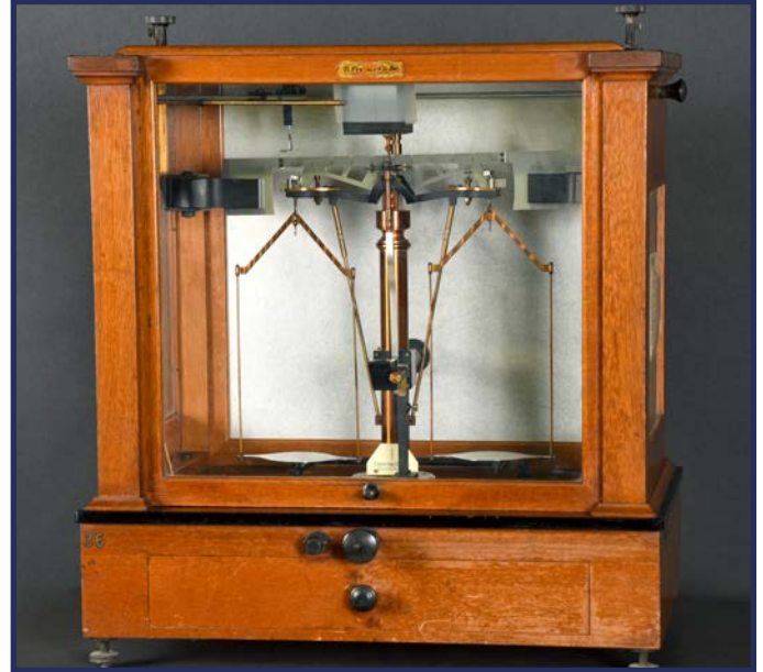
Christian Becker Projection Reading Analytical Balance No. 911, circa 1950, used at Union Carbide by Lab Technician Steven Lawrence Marcum (1947-2017) Donated by Marie Marcum of Charleston, West Virginia
